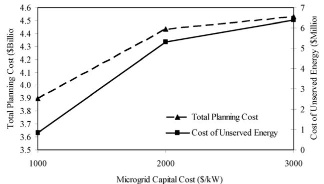
Fig. 3. Total planning cost and cost of unserved energy as a function of microgrid capital cost.
