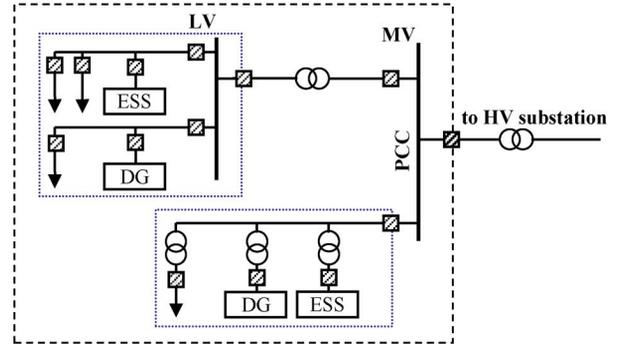
Fig. 1. Typical microgrid architecture (DG: distributed generation, ESS: energy storage system, PCC: point of common coupling).
