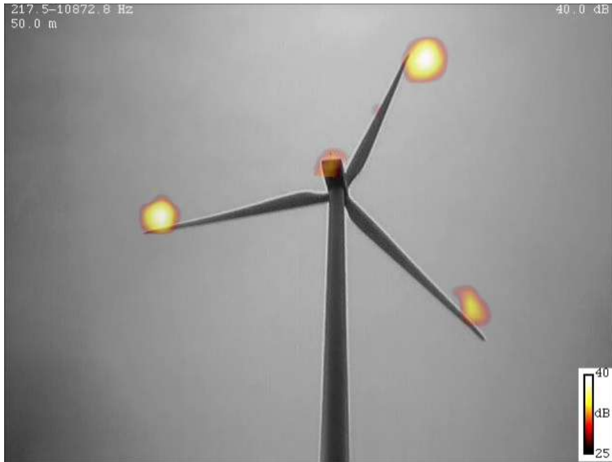
Figure 185: Beamform map of the GE 1.5 MW wind turbine using TIDY at a particular instant of time during its rotation.
