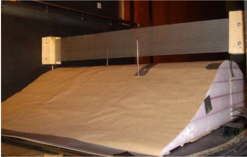
Figure 355: Photograph of Porous plate and surface shape in wind tunnel.
