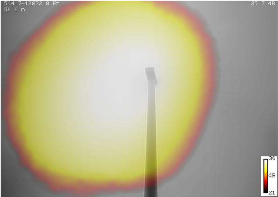
Figure 183: Beamform map of the GE 1.5 MW wind turbine using DAS.
