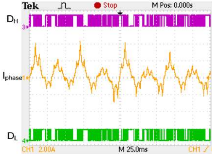
Figure 139: Phase current and change of duty cycle
