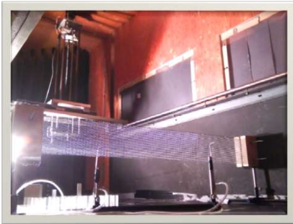
Figure 352: Photograph depicting porous plate set-up in wind tunnel
