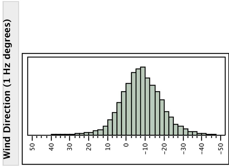
Figure 4 The distribution of yaw angles with respect to the free wind, as measured by the OCS. The turbine is under legacy control. The distribution is roughly symmetric. The mean of the distribution is -7.8 degrees, with a standard deviation of 11.8 degrees.
