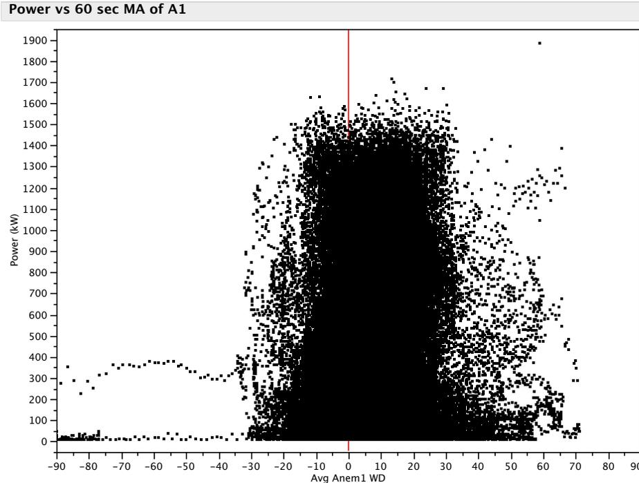
Figure 2 A scatter plot of power vs. post-rotor wind angle measured by the anemometer. The data is not symmetric, with the center of the distribution being offset by ~10 degrees.
