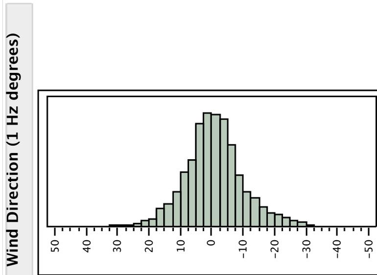
Figure 6 The distribution of yaw angles, based upon the free wind in front of the turbine as measured by the OCS. The distribution is shifted, with the mean now at -0.9 degrees. The distribution of yaw angle is substantially narrower, with standard deviation now down to 9.7 degrees.
