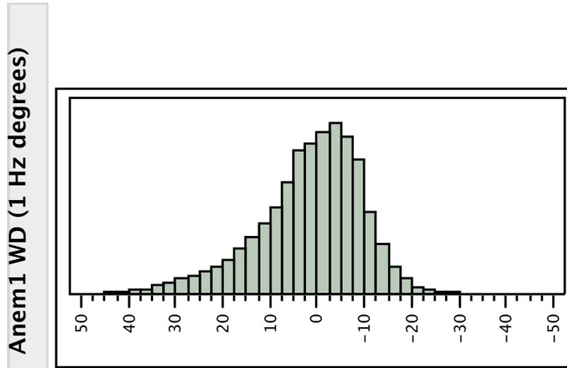
Figure 3 The measured distribution of wind angles, as measured in the post-rotor wind flow. The bottom is degrees. The distribution has mean and median of 1.55 and 0 degrees, respectively. The standard deviation is 11.3 degrees.
