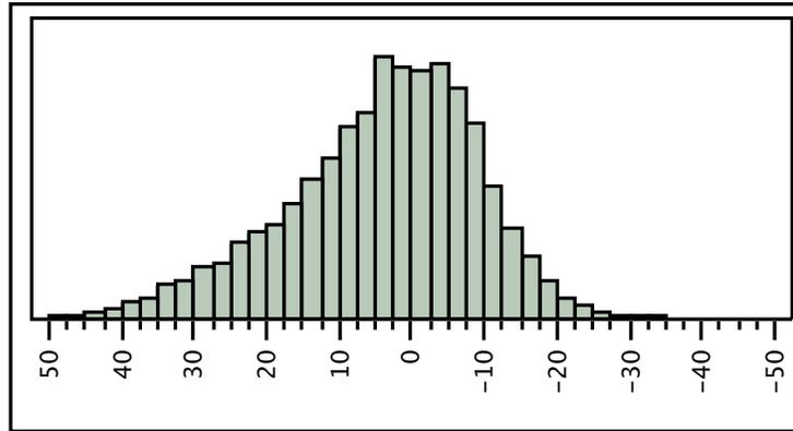
Figure 5 The distribution of yaw angles, measured in the post-rotor flow by the sonic anemometer. The distribution is still asymmetry, as before, but the mean of the distribution has been shifted to 4.2 degrees. Under OCS control the distribution measured by the anemometer significantly broadens, with standard deviation increasing to 13.6 degrees.
