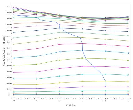
Figure 8 A contour plot showing curves of constant wind speed. The blue line indicates the angle of maximum power production. Each integer unit on the X-axis corresponds to 10 degrees, indicating that the angle of maximum power varies substantially.
