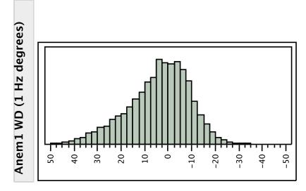
Figure 5 The distribution of yaw angles, measured in the post-rotor flow by the sonic anemometer. The distribution is still asymmetry, as before, but the mean of the distribution has been shifted to 4.2 degrees. Under OCS control the distribution measured by the anemometer significantly broadens, with standard deviation increasing to 13.6 degrees.
