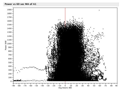
Figure 2 A scatter plot of power vs. post-rotor wind angle measured by the anemometer. The data is not symmetric, with the center of the distribution being offset by  $\sim 10$  degrees.
