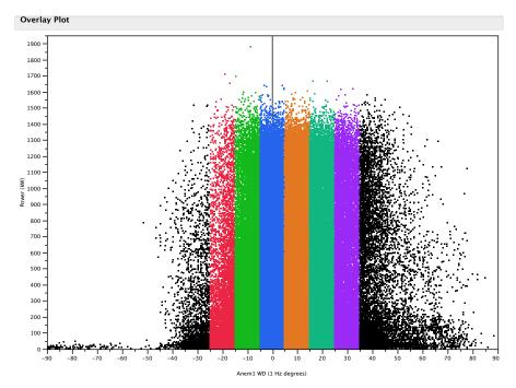
Figure 7 The scatterplot of wind angle as measured by the post-rotor anemometer. The color-coding of the data points indicates the angle bins.
