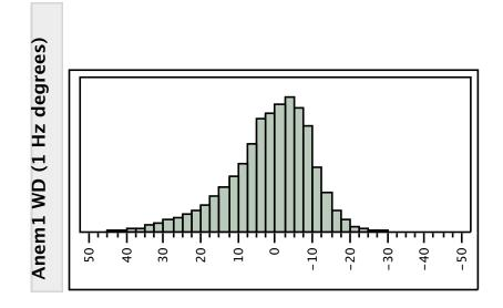
Figure 3 The measured distribution of wind angles, as measured in the post-rotor wind flow. The bottom is degrees. The distribution has mean and median of 1.55 and 0 degrees, respectively. The standard deviation is 11.3 degrees.
