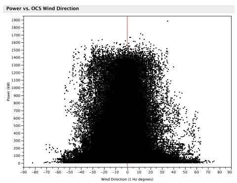
Figure 1 A scatter plot of the output power of the turbine vs. wind angle as measured by the OCS.
