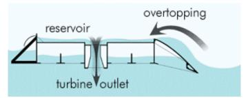
Figure 9. Ocean Wave Turbine
