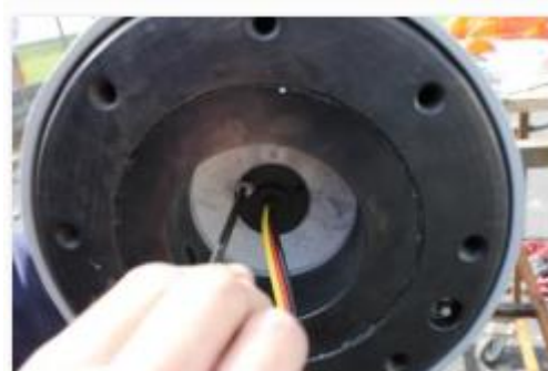
Use Fixings Provided to Secure Slip Ring
