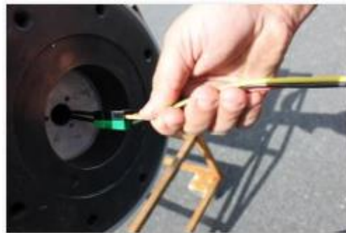
Connect to Rotary Side of Slip Ring
