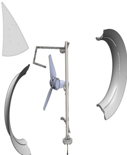
Rotor Assembly, Tail Fin Assembly & Enhancement Unit Halves Exploded Assembly
