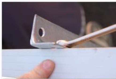
You may use Spanner to secure Nuts But Tighten Later to Correct Torque Settings. Don't Over Tighten
