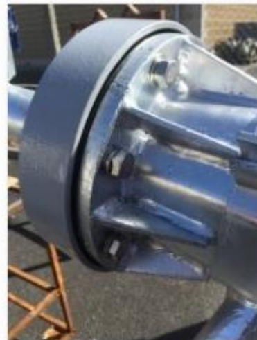
Use Bolts and Spring Washers to Fix Bearing to the Top of Flange on Tower
