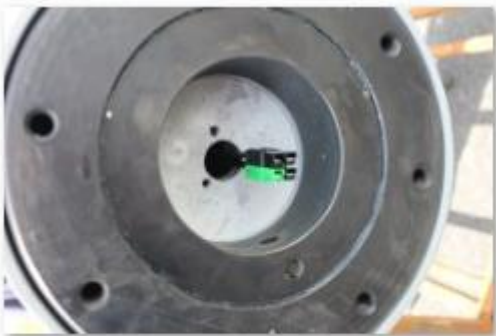
Extract Connection Terminals for connection to the Slip Ring
