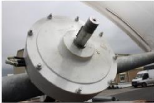
Ready Sanho 300W Generator for Receiving Rotor
