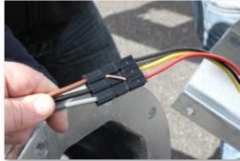
Secure with Staple Shaped Copper Wire Fasteners as Shown
