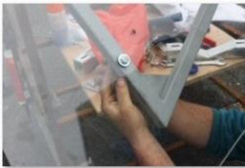
Fit Tail Fin to Tail Fin Bracket and Hand Tighten
