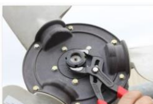
After Mounting Rotor Boss and Hub tighten Holding on Nuts
