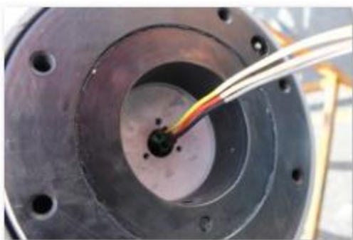
Re-insert Connection Terminals into Pole
