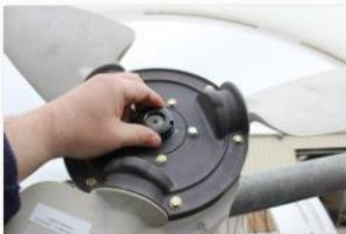
Align Shaft Key with Key Way and Mount Rotor Boss and Hub and Hand Tighten
