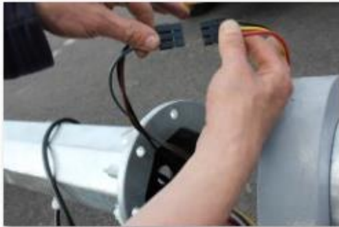
Connect Terminals of Slip Ring to Generator Wiring Loom from Tower
