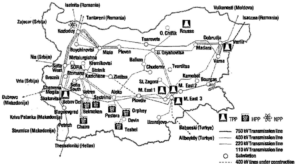
Fig. 1. Map of the Electric Power Network of Bulgaria
