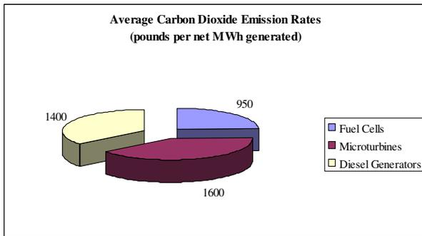
Fig. 2 (a). Comparative plot of average carbon dioxide emission rates
