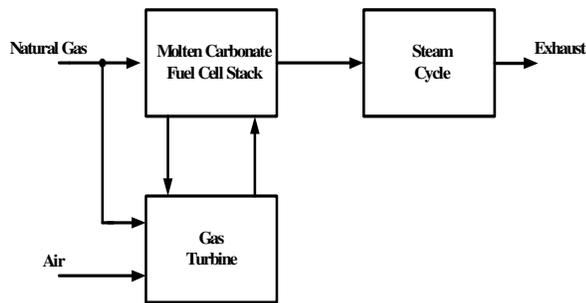
Fig. 4. A MCFC-hybrid power cycle
