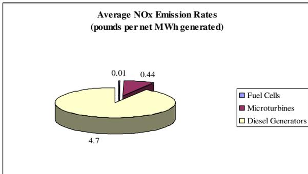
Fig. 2 (b). Comparative plot of average NO<sub>x</sub> emission rates
