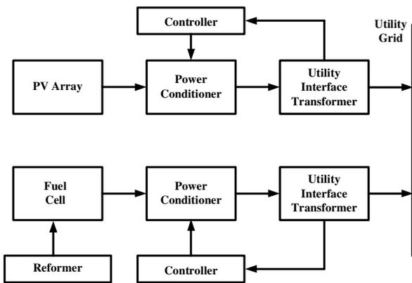
Fig. 6. Schematic block diagram of a fuel cell-PV hybrid system.
