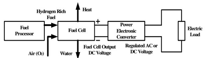
Fig. 1. Block diagram of a fuel cell-based power system
