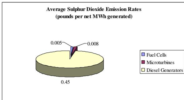
Fig. 2 (c). Comparative plot of average SO<sub>x</sub> emission rates
