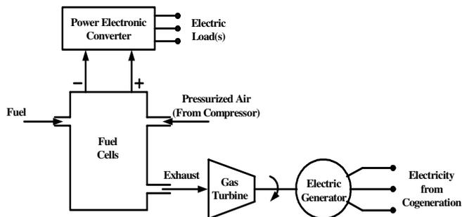
Fig. 5. Typical layout of a SOFC-based cogeneration plant
