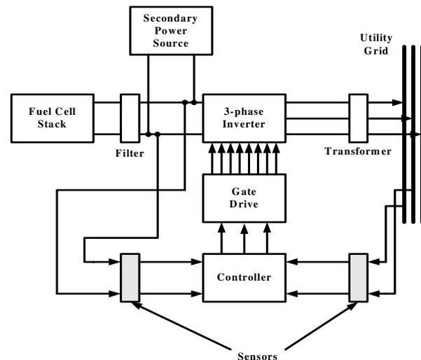
Fig. 7. Utility interface with a fuel cell system
