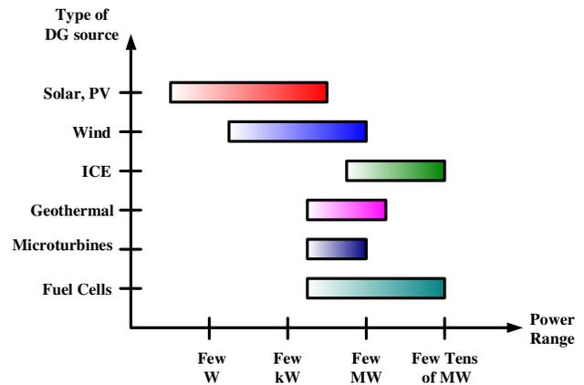
Fig. 3. Power ranges of DG technologies
