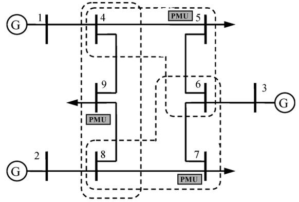
Fig. 2. Observability with no PMUs at zero-injection buses.
