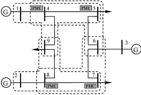
Fig. 3. Observability considering the loss of a single measurement.
