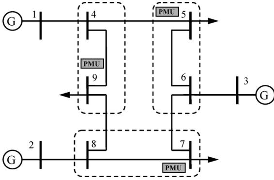
Fig. 5. Observability considering measurement limitations.
