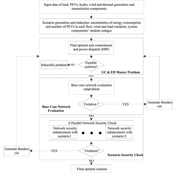
Fig. 1. Proposed Stochastic SCUC with PEV integration in power systems.
