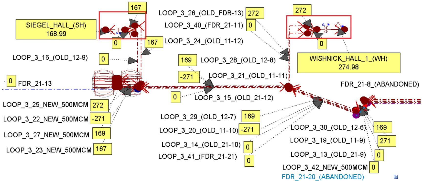
In the section 1, as we can see from the snapshot of the network, the power comes from the 2 feeders connected to the **North Substation**. The yellow boxes represent the following (from top)
