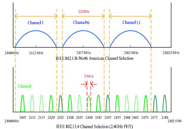
Fig. 5. ZigBee and WiFi channels in the 2.4 GHz band
