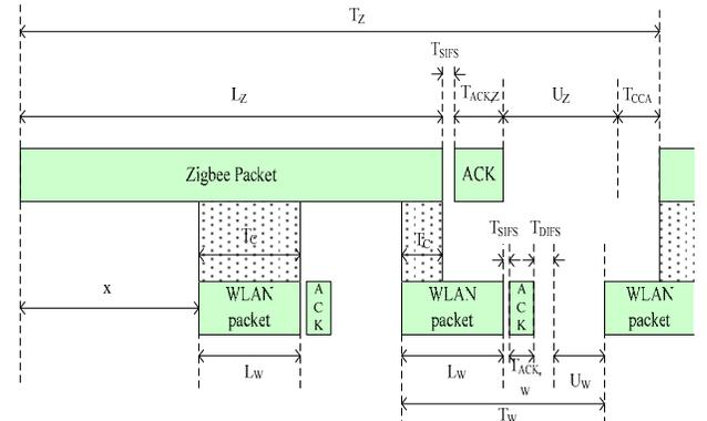
Fig. 2. IEEE 802.11b and IEEE 802.15.4 Interference Model [2]
