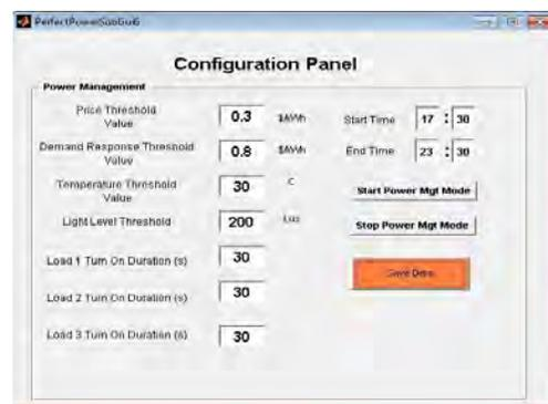
Fig. 10. System configuration panel
