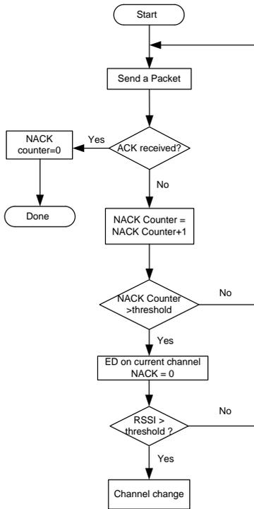
Fig.4. Flowchart of interference detection
