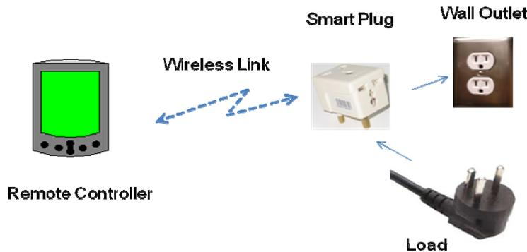
Figure 7: Smart Plug System
