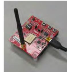
Fig. 3. Meshnetics Meshbean2 Zigbee mote
