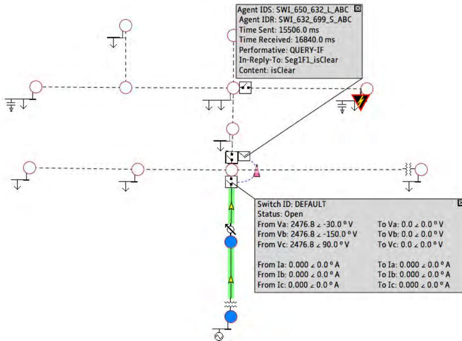
Figure 3: Java FX Display with Isolated Fault and Agent Messages at T=1.6840 s
