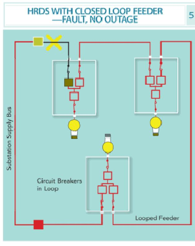
The key innovation in the HRDS is that the entire loop remains energized during the fault scenario presented. Additional equipment is required in an HRDS beyond the typical equipment in a traditional radial system with manual switches.
