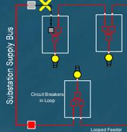
Breakers Isolate Fault to Only One Section
