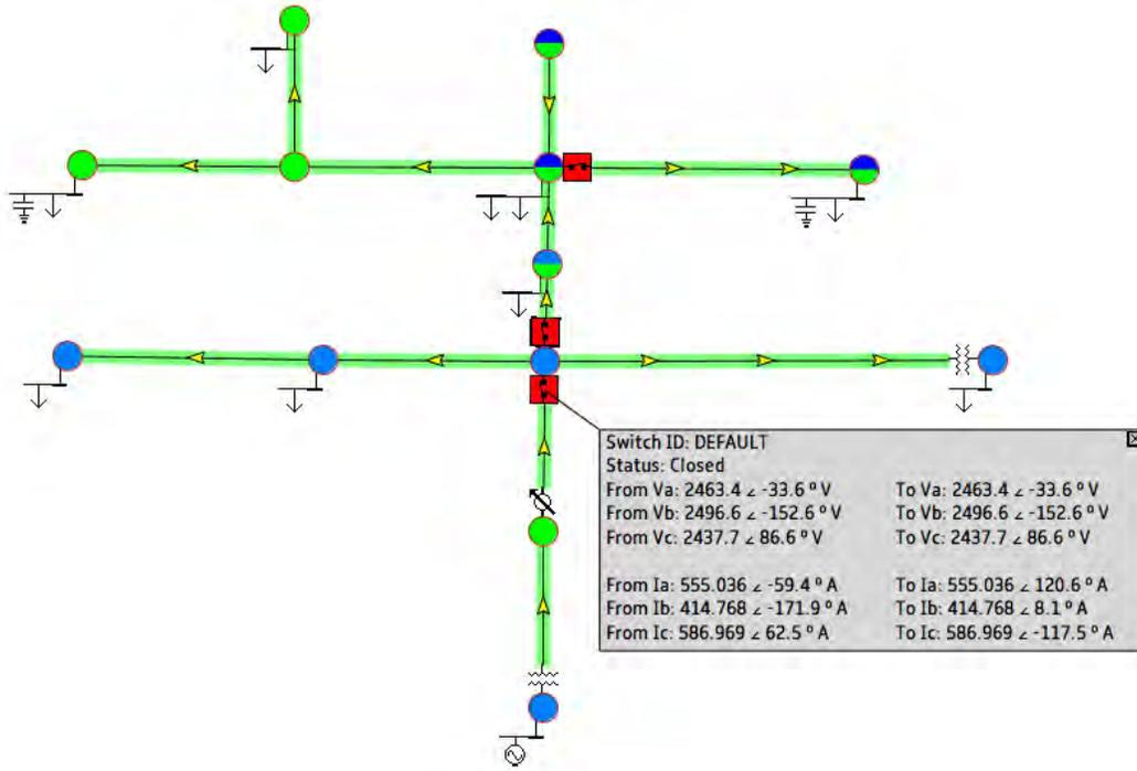
Figure 1: Java FX Display with Closed Switch Info Box at T=0 s
