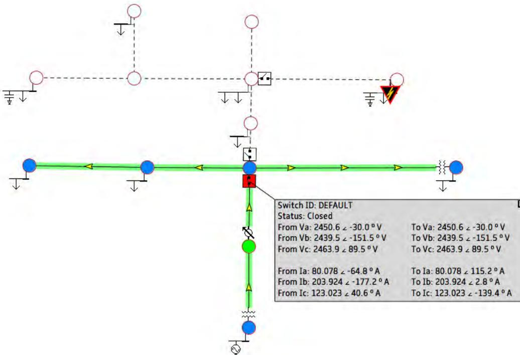
Figure 5: Java FX Display with Partially Restored Feeder at T=1.8178 s
