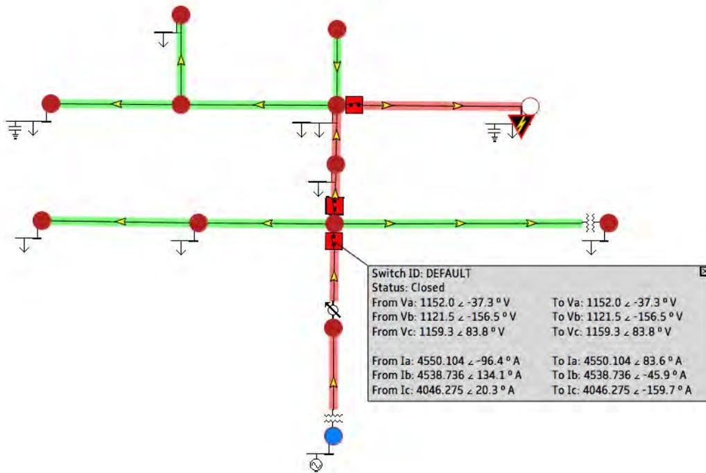
Figure 2: Java FX Display with Fault at T=1.0 s
