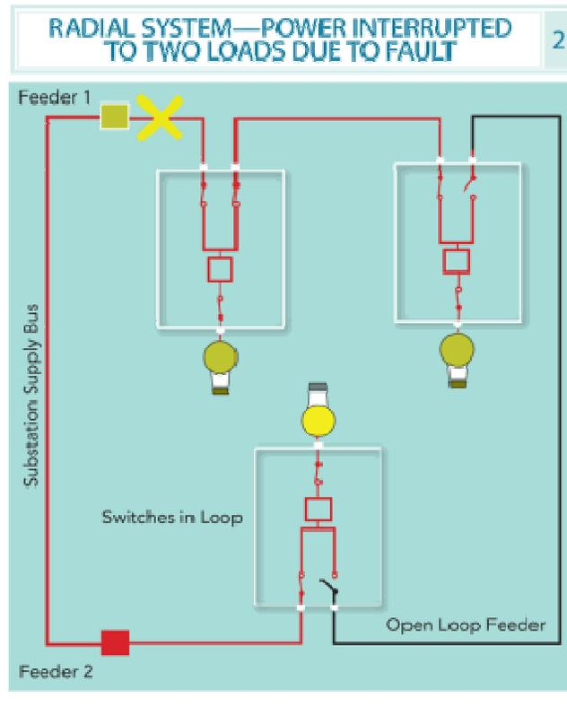
Following power loss, an electrician would be notified of the outage. In a typical distribution system, the steps required to restore power to all customers, and the time required for each step, are shown below:
