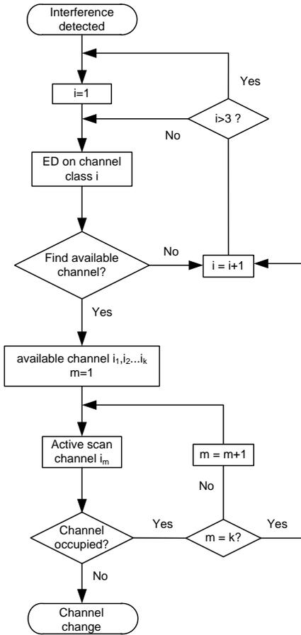
Fig.6. Flowchart of the Interference Avoidance
