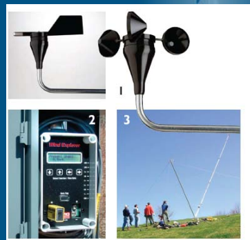
1) Anemometer and Wind Direction Vane 2) Datalogger 3) Met Tower
