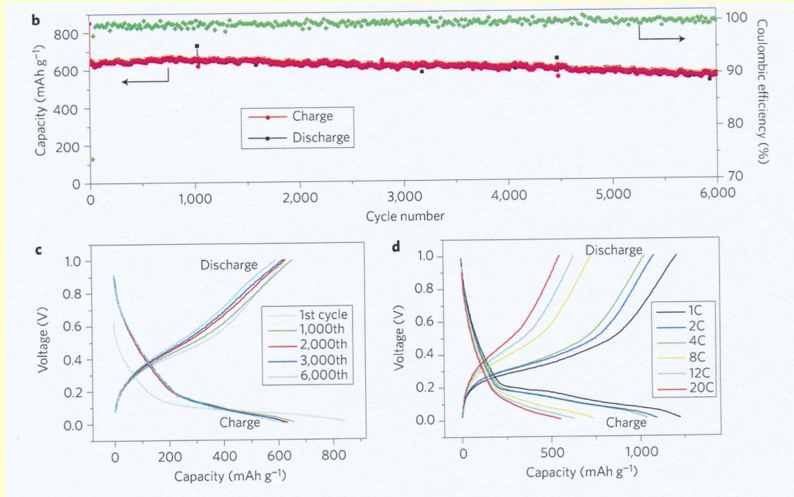
Charge/discharge rate in 12C over 6,000 cycles with a capacity of 600 mAh/g.
