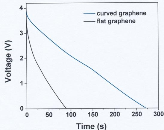
Discharge curves of curved graphene vs flat graphene electrodes
