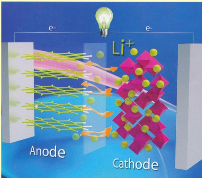
Li-ion batteries store energy through redox reactions of the host materials induced by Li-ion intercalation & deintercalation.
