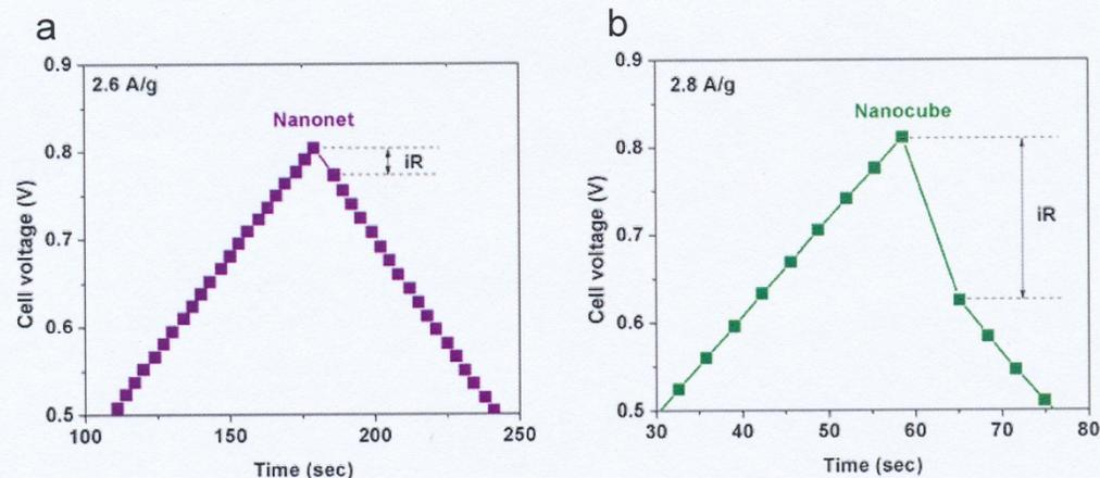
Nanonet has better rate capability and higher coulombic efficiency than nanocube.
