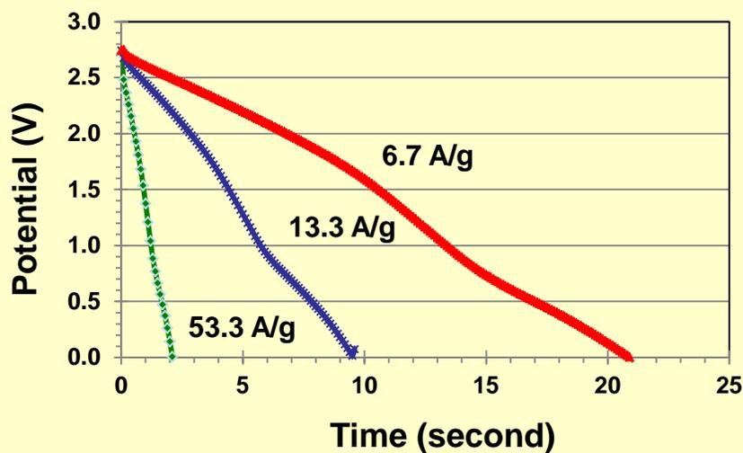
A comparison of galvanostatic discharge curves for 3 different current densities as indicated
