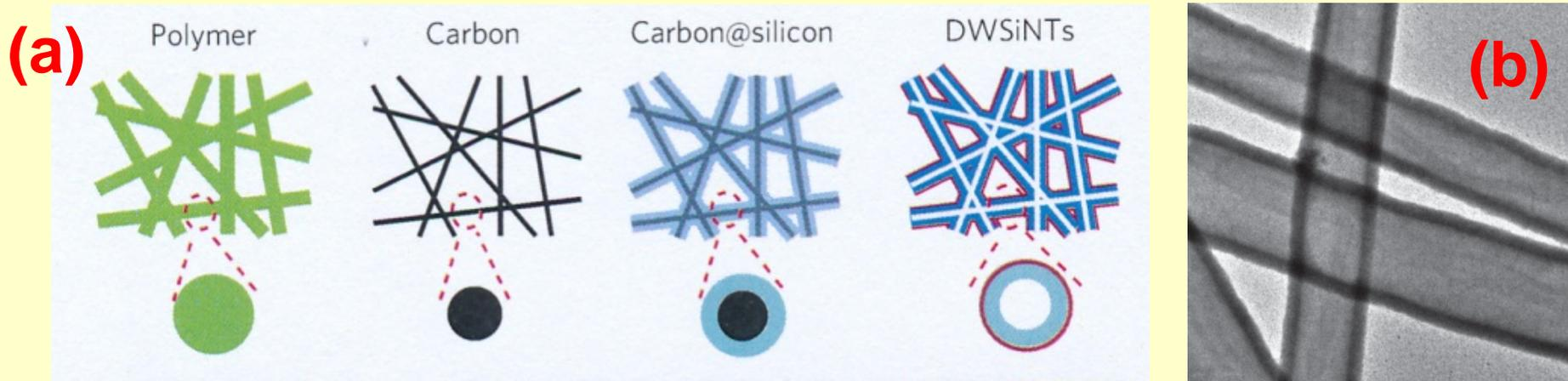
Fabrication process for DWSiNTs: (i) polyacrylonitrile (PAN) fibers via electrospinning; (ii) carbonization of PAN fibers at 500°C; (iii) Si coating of 30 nm thick via SiH<sub>4</sub> chemical vapour deposition (CVD); (iv) carbon core removal at 500°C in air and oxidation of the Si nanotube surface.
