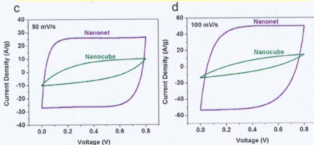
Nanonet has excellent “rectangular-shape” cyclic voltammograms, whereas nanocube has “distorted” CV curves.
