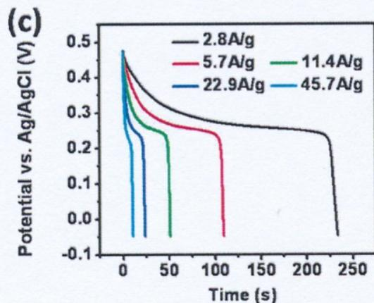
CV and galvanostatic discharge curves of nano-Ni(OH)<sub>2</sub> on graphene
