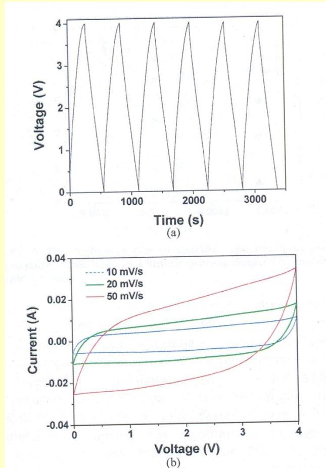
Galvanostatic charge-discharge curves of a curved graphene electrode (1 A/g, IL electrolyte)
