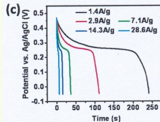
CV and galvanostatic discharge curves of nano-Ni(OH)<sub>2</sub> physically mixed with graphene
