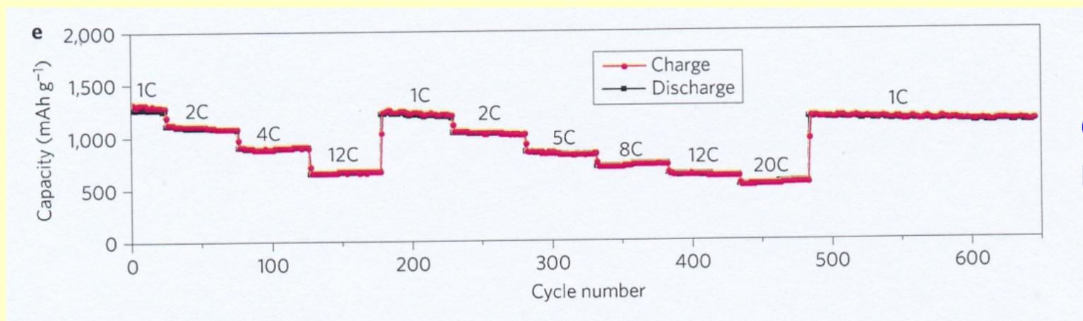
Capacity at 1,250 mAh/g in 1C
