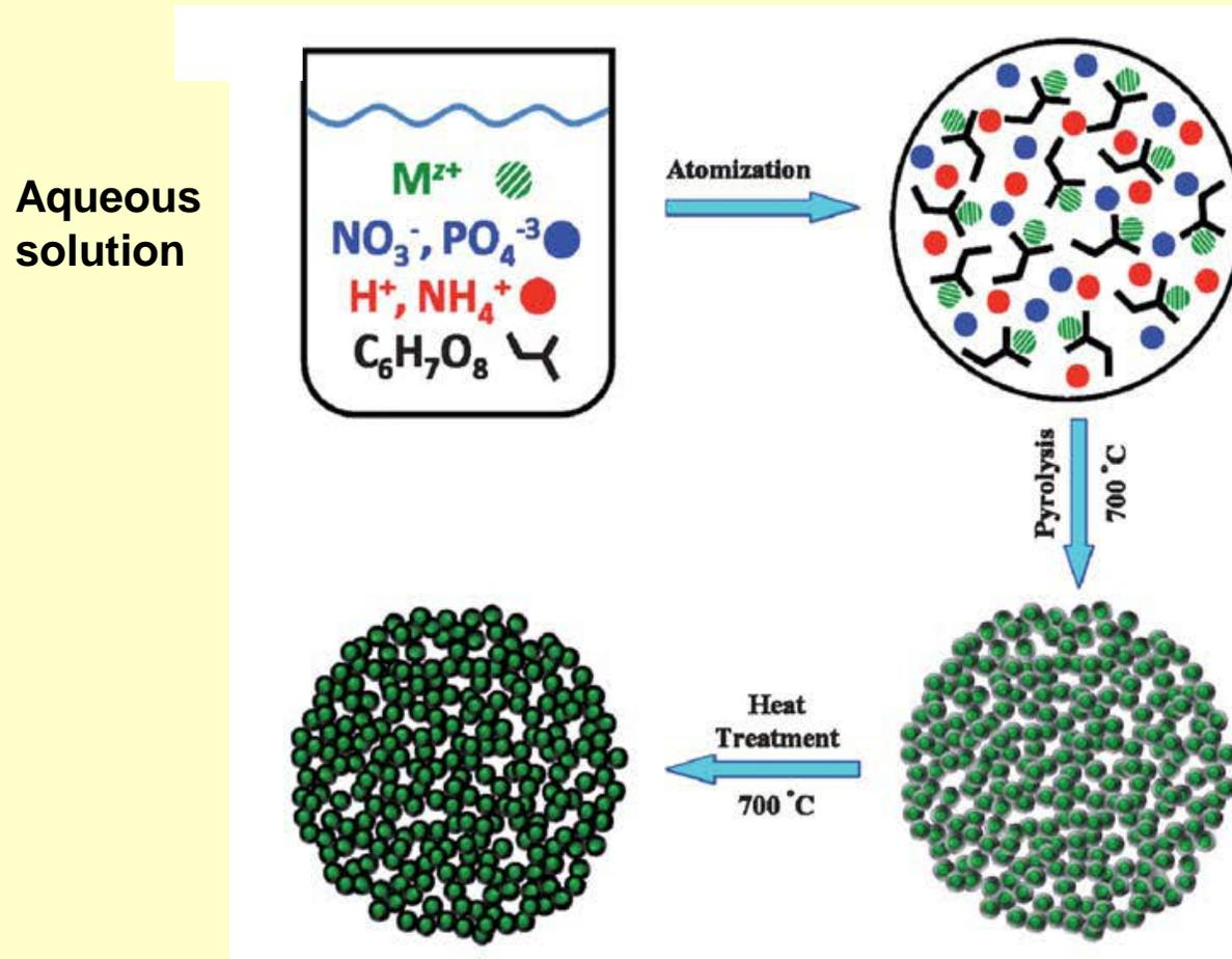
Steps for the formation porous  $\text{LiFePO}_4/\text{C}$  particles via spray pyrolysis.
