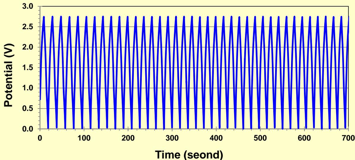
Galvanostatic charge/discharge cycling curves with a current density of 13.3 A/g.
