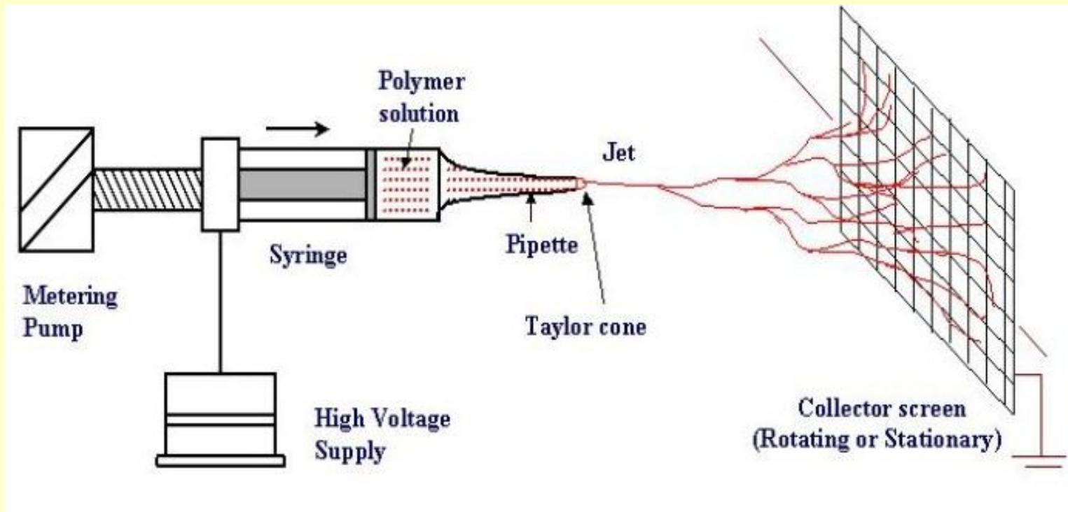
**Electrospinning uses an electrical charge to draw very fine fibers from liquid.**
