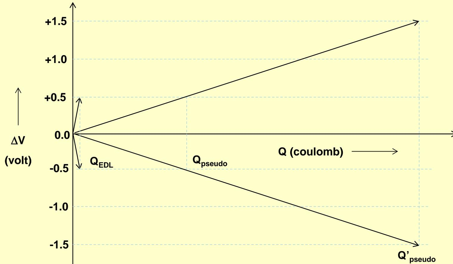
Schematic of the storage capacity: (i) pseudocapacitance,  $Q_{pseudo}$ , can increase the energy density by ~ 10 times, (ii) pseudocapacitance along with increasing the cell voltage from 1 to 3 V,  $Q'_{pseudo}$ , can increase the energy density by ~30 times.
