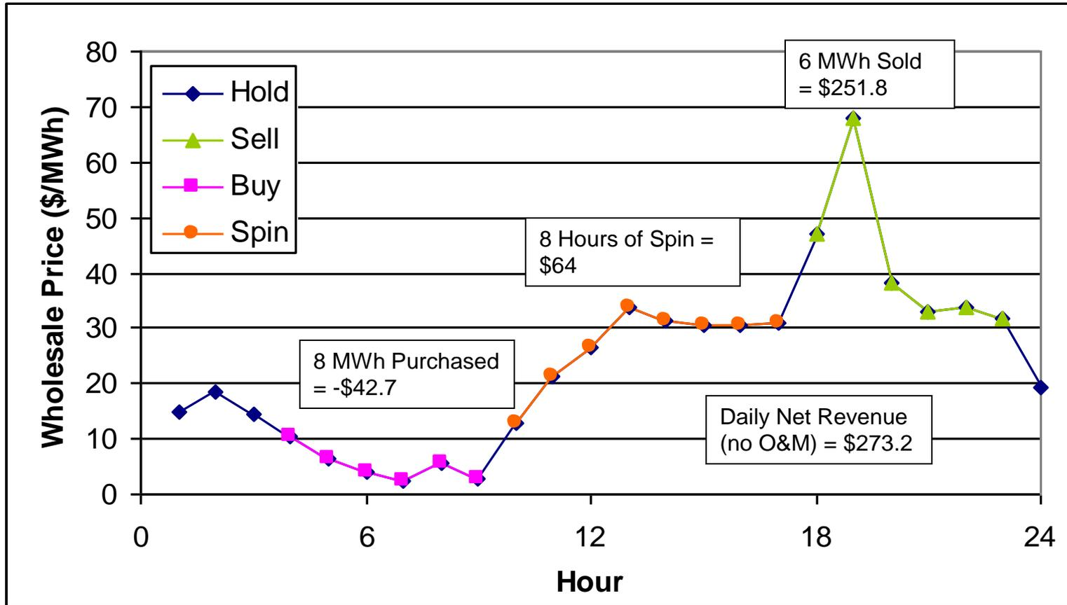
1 MW, 6 MWh Device, 75% efficiency
