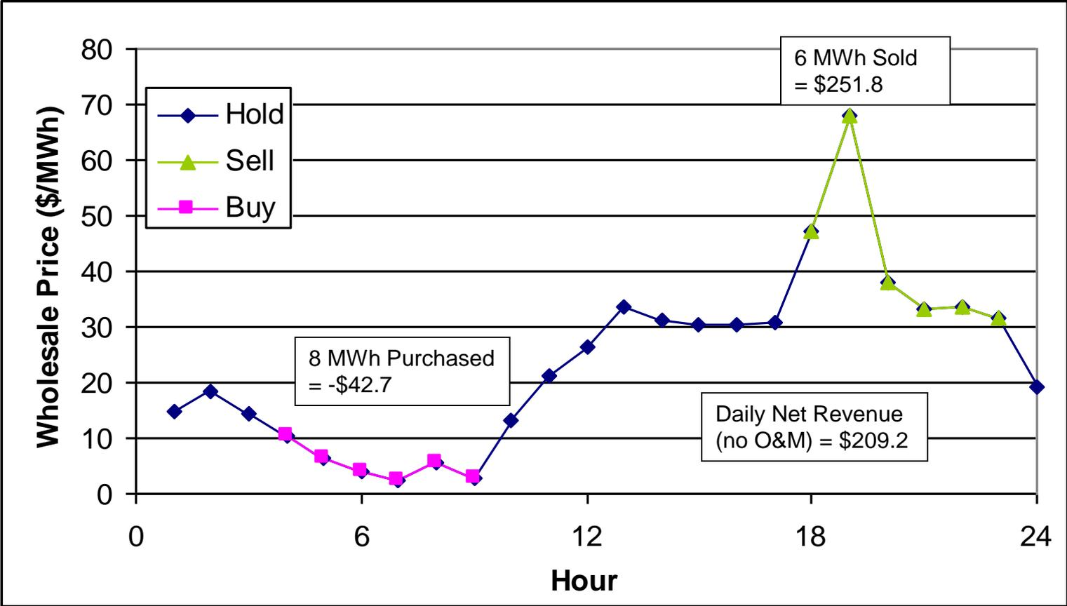
1 MW, 6 MWh Device, 75% efficiency
