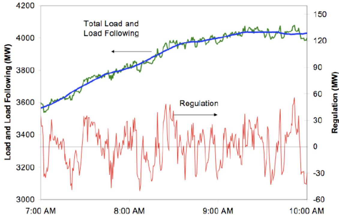
System load following and regulation. Regulation (red) is the fast fluctuating component of total load (green) while load following (blue) is the slower trend
