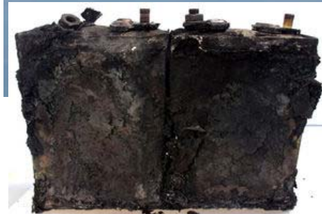
Cell#6 short circuit 500+degF 'issue'
