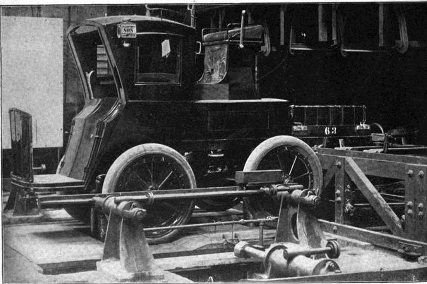
ELECTRIC HANSOM, SHOWING HYDRAULIC RAM FOR SIDE ALIGNMENT AND BATTERY IN POSITION FOR LOADING.
