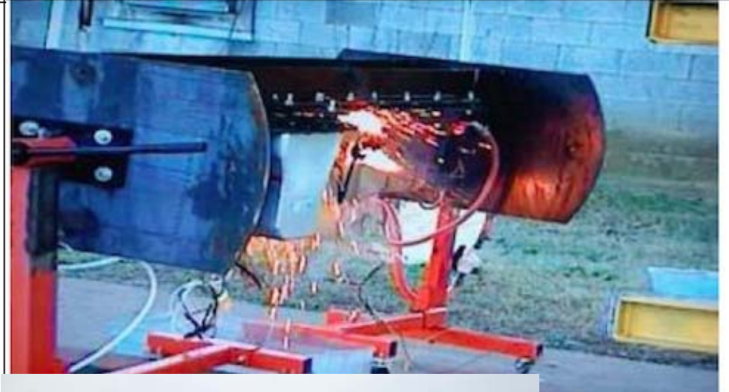
Figure 5.04 Battery 3 Arcing Event
